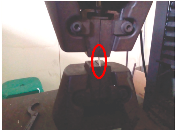
Figure 2. Tensile strength examination using the Shimidzu Autograph AG instrument
